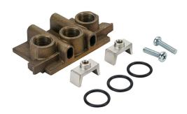
NITRA air manifold inlet, aluminum alloy, 145 psi (10 bar) maximum operating pressure, G3/8 female BSPP inlet(s), G3/8 female BSPP exhaust(s). For use with ISO 5599/1 size 1 manifolds.
