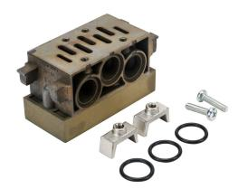
NITRA air manifold base, aluminum alloy, 145 psi (10 bar) maximum operating pressure, 1/4in female NPT outlet(s), bottom orientation. For use with ISO 5599/1 size 1 solenoid valves.
