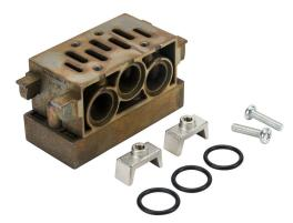
NITRA air manifold base, aluminum alloy, 145 psi (10 bar) maximum operating pressure, G1/4 female BSPP outlet(s), bottom orientation. For use with ISO 5599/1 size 1 solenoid valves.
