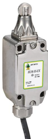
IDEM safety limit switch, hazardous location rated, plunger with stainless steel roller, (2) N.C. safety output(s), (2) N.O. monitoring output(s), slow action break before make, 316 stainless steel, pigtail.
