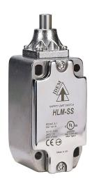
IDEM safety limit switch, stainless steel plunger, (1) N.C. safety output(s), (1) N.O. monitoring output(s), snap action, 316 stainless steel, (1) 1/2in female NPT conduit.
