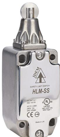
IDEM safety limit switch, plunger with stainless steel roller, (2) N.C. safety output(s), (2) N.O. monitoring output(s), slow action break before make, 316 stainless steel, (1) 1/2in female NPT conduit.
