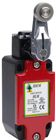
IDEM safety limit switch, side rotary lever with stainless steel roller, (2) N.C. safety output(s), (2) N.O. monitoring output(s), slow action break before make, die-cast zinc aluminum, (1) 1/2in female NPT conduit.
