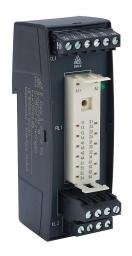
Dold relay socket, 14-pin, 35mm DIN rail mount, LED indicator(s), diode protection. For use with OA5612 series relays.
