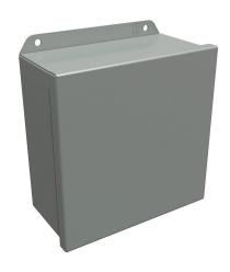
Hammond enclosure, NEMA 3R/4/12/13, 8 x 8 x 4in (HxWxD), wall mount, carbon steel, ANSI 61 gray, powder coat finish, single-door, stainless steel clamps.
