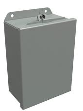
Hammond enclosure, NEMA 3R/4/12/13,  $8 \times 6 \times 3.5$  in (HxWxD), wall mount, carbon steel, ANSI 61 gray, powder coat finish, lift-off cover, stainless steel clamps.
