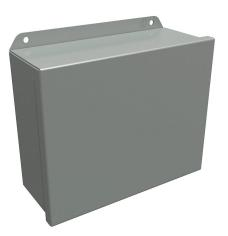
Hammond enclosure, NEMA 3R/4/12/13, 8 x 10 x 4in (HxWxD), wall mount, carbon steel, ANSI 61 gray, powder coat finish, single-door, stainless steel clamps.
