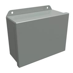
Hammond enclosure, NEMA 3R/4/12/13, 6 x 8 x 3in (HxWxD), wall mount, carbon steel, ANSI 61 gray, powder coat finish, single-door, stainless steel clamps.
