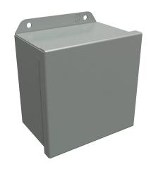
Hammond enclosure, NEMA 3R/4/12/13, 6 x 6 x 4in (HxWxD), wall mount, carbon steel, ANSI 61 gray, powder coat finish, single-door, stainless steel clamps.
