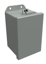
Hammond enclosure, NEMA 3R/4/12/13, 6 x 4 x 4in (HxWxD), wall mount, carbon steel, ANSI 61 gray, powder coat finish, lift-off cover, stainless steel clamps.
