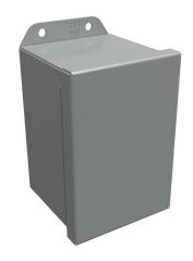
Hammond enclosure, NEMA 3R/4/12/13, 6 x 4 x 4in (HxWxD), wall mount, carbon steel, ANSI 61 gray, powder coat finish, single-door, stainless steel clamps.
