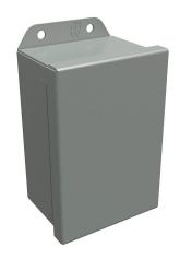
Hammond enclosure, NEMA 3R/4/12/13, 6 x 4 x 3in (HxWxD), wall mount, carbon steel, ANSI 61 gray, powder coat finish, single-door, stainless steel clamps.
