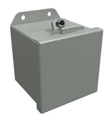
Hammond enclosure, NEMA 3R/4/12/13, 4 x 4 x 4in (HxWxD), wall mount, carbon steel, ANSI 61 gray, powder coat finish, lift-off cover, stainless steel clamps.
