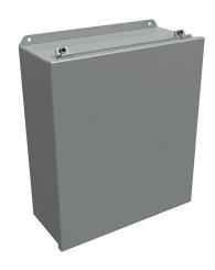
Hammond enclosure, NEMA 3R/4/12/13, 16 x 14 x 6in (HxWxD), wall mount, carbon steel, ANSI 61 gray, powder coat finish, lift-off cover, stainless steel clamps.
