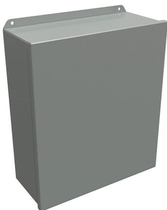
Hammond enclosure, NEMA 3R/4/12/13, 16 x 14 x 6in (HxWxD), wall mount, carbon steel, ANSI 61 gray, powder coat finish, single-door, stainless steel clamps.
