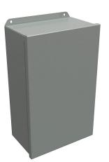
Hammond enclosure, NEMA 3R/4/12/13,  $16 \times 10 \times 6in$  (HxWxD), wall mount, carbon steel, ANSI 61 gray, powder coat finish, single-door, stainless steel clamps.
