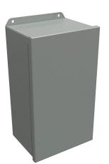
Hammond enclosure, NEMA 3R/4/12/13, 14 x 8 x 6in (HxWxD), wall mount, carbon steel, ANSI 61 gray, powder coat finish, single-door, stainless steel clamps.
