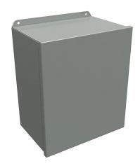
Hammond enclosure, NEMA 3R/4/12/13,  $14 \times 12 \times 8$ in (HxWxD), wall mount, carbon steel, ANSI 61 gray, powder coat finish, single-door, stainless steel clamps.
