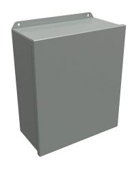
Hammond enclosure, NEMA 3R/4/12/13, 14 x 12 x 6in (HxWxD), wall mount, carbon steel, ANSI 61 gray, powder coat finish, single-door, stainless steel clamps.
