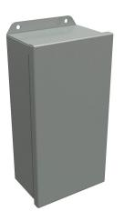
Hammond enclosure, NEMA 3R/4/12/13, 12 x 6 x 4in (HxWxD), wall mount, carbon steel, ANSI 61 gray, powder coat finish, single-door, stainless steel clamps.
