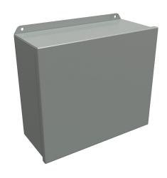
Hammond enclosure, NEMA 3R/4/12/13, 12 x 14 x 6in (HxWxD), wall mount, carbon steel, ANSI 61 gray, powder coat finish, single-door, stainless steel clamps.
