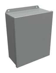
Hammond enclosure, NEMA 3R/4/12/13, 12 x 10 x 5in (HxWxD), wall mount, carbon steel, ANSI 61 gray, powder coat finish, single-door, stainless steel clamps.
