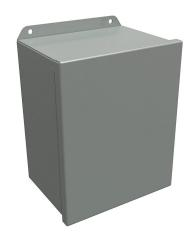
Hammond enclosure, NEMA 3R/4/12/13, 10 x 8 x 6in (HxWxD), wall mount, carbon steel, ANSI 61 gray, powder coat finish, single-door, stainless steel clamps.
