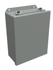
Hammond enclosure, NEMA 3R/4/12/13,  $10 \times 8 \times 4$  in (HxWxD), wall mount, carbon steel, ANSI 61 gray, powder coat finish, lift-off cover, stainless steel clamps.
