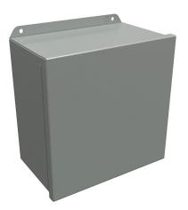
Hammond enclosure, NEMA 3R/4/12/13,  $10 \times 10 \times 6$  in (HxWxD), wall mount, carbon steel, ANSI 61 gray, powder coat finish, single-door, stainless steel clamps.
