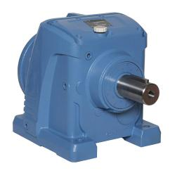
IronHorse heavy-duty helical gearbox, 60:1 ratio, 182TC-Face input, inline, 2.125in diameter output shaft, nominal 3hp at 1.0 SF, 6030 lb-in mechanical output torque, Type-87 frame, cast iron housing, foot mount.
