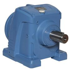
IronHorse heavy-duty helical gearbox, 40:1 ratio, 182/4TC-Face input, inline, 2.125in diameter output shaft, nominal 5hp at 1.0 SF, 6240 lb-in mechanical output torque, Type-87 frame, cast iron housing, foot mount.
