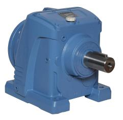
IronHorse heavy-duty helical gearbox, 30:1 ratio, 182/4TC-Face input, inline, 2.125in diameter output shaft, nominal 5hp at 1.0 SF, 5180 lb-in mechanical output torque, Type-87 frame, cast iron housing, foot mount.
