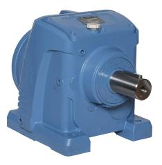
IronHorse heavy-duty helical gearbox, 20:1 ratio, 182/4TC-Face input, inline, 2.125in diameter output shaft, nominal 5hp at 1.0 SF, 3280 lb-in mechanical output torque, Type-87 frame, cast iron housing, foot mount.
