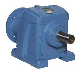
IronHorse heavy-duty helical gearbox, 5:1 ratio, 254/6TC-Face input, inline, 2.125in diameter output shaft, nominal 15hp at 1.0 SF, 2390 lb-in mechanical output torque, Type-87 frame, cast iron housing, foot mount.
