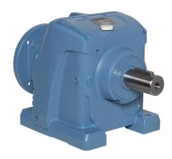
IronHorse heavy-duty helical gearbox, 5:1 ratio, 213/5TC-Face input, inline, 2.125in diameter output shaft, nominal 10hp at 1.0 SF, 1590 lb-in mechanical output torque, Type-87 frame, cast iron housing, foot mount.
