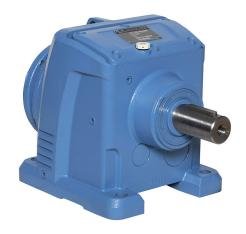
IronHorse heavy-duty helical gearbox, 60:1 ratio, 145TC-Face input, inline, 1.625in diameter output shaft, nominal 2hp at 1.0 SF, 3770 lb-in mechanical output torque, Type-77 frame, cast iron housing, foot mount.
