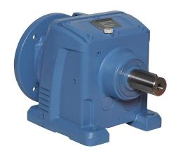
IronHorse heavy-duty helical gearbox, 40:1 ratio, 182/4TC-Face input, inline, 1.625in diameter output shaft, nominal 3hp at 1.0 SF, 3850 lb-in mechanical output torque, Type-77 frame, cast iron housing, foot mount.
