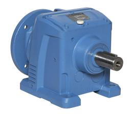
IronHorse heavy-duty helical gearbox, 30:1 ratio, 182/4TC-Face input, inline, 1.625in diameter output shaft, nominal 3hp at 1.0 SF, 3130 lb-in mechanical output torque, Type-77 frame, cast iron housing, foot mount.
