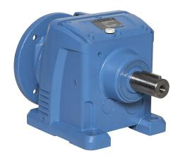
IronHorse heavy-duty helical gearbox, 30:1 ratio, 182/4TC-Face input, inline, 1.625in diameter output shaft, nominal 3hp at 1.0 SF, 3130 lb-in mechanical output torque, Type-77 frame, cast iron housing, foot mount.
