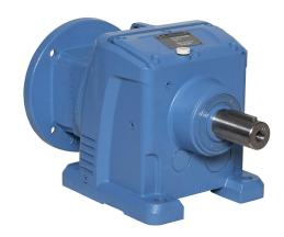
IronHorse heavy-duty helical gearbox, 10:1 ratio, 213/5TC-Face input, inline, 1.625in diameter output shaft, nominal 7.5hp at 1.0 SF, 2760 lb-in mechanical output torque, Type-77 frame, cast iron housing, foot mount.
