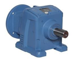
IronHorse heavy-duty helical gearbox, 5:1 ratio, 213/5TC-Face input, inline, 1.625in diameter output shaft, nominal 7.5hp at 1.0 SF, 1210 lb-in mechanical output torque, Type-77 frame, cast iron housing, foot mount.
