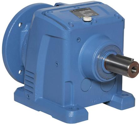
IronHorse heavy-duty helical gearbox, 5:1 ratio, 182/4TC-Face input, inline, 1.625in diameter output shaft, nominal 5hp at 1.0 SF, 800 lb-in mechanical output torque, Type-77 frame, cast iron housing, foot mount.
