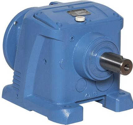
IronHorse heavy-duty helical gearbox, 40:1 ratio, 145TC-Face input, inline, 1.375in diameter output shaft, nominal 2hp at 1.0 SF, 2690 lb-in mechanical output torque, Type-67 frame, cast iron housing, foot mount.
