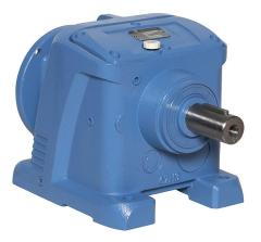
IronHorse heavy-duty helical gearbox, 30:1 ratio, 145TC-Face input, inline, 1.375in diameter output shaft, nominal 2hp at 1.0 SF, 1880 lb-in mechanical output torque, Type-67 frame, cast iron housing, foot mount.
