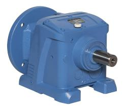
IronHorse heavy-duty helical gearbox, 20:1 ratio, 182TC-Face input, inline, 1.375in diameter output shaft, nominal 3hp at 1.0 SF, 2160 lb-in mechanical output torque, Type-67 frame, cast iron housing, foot mount.
