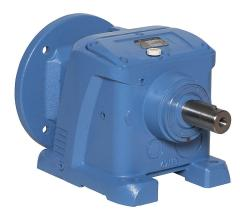
IronHorse heavy-duty helical gearbox, 15:1 ratio, 182TC-Face input, inline, 1.375in diameter output shaft, nominal 3hp at 1.0 SF, 1560 lb-in mechanical output torque, Type-67 frame, cast iron housing, foot mount.
