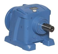
IronHorse heavy-duty helical gearbox, 15:1 ratio, 145TC-Face input, inline, 1.375in diameter output shaft, nominal 2hp at 1.0 SF, 1040 lb-in mechanical output torque, Type-67 frame, cast iron housing, foot mount.
