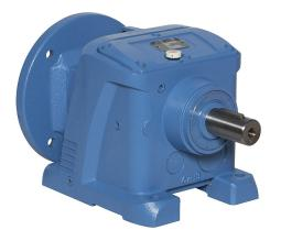
IronHorse heavy-duty helical gearbox, 10:1 ratio, 182/4TC-Face input, inline, 1.375in diameter output shaft, nominal 5hp at 1.0 SF, 1670 lb-in mechanical output torque, Type-67 frame, cast iron housing, foot mount.
