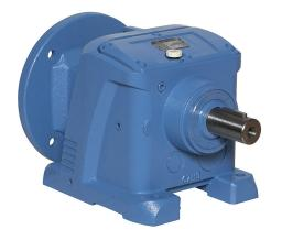
IronHorse heavy-duty helical gearbox, 5:1 ratio, 182/4TC-Face input, inline, 1.375in diameter output shaft, nominal 5hp at 1.0 SF, 880 lb-in mechanical output torque, Type-67 frame, cast iron housing, foot mount.
