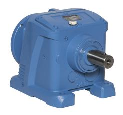
IronHorse heavy-duty helical gearbox, 5:1 ratio, 145TC-Face input, inline, 1.375in diameter output shaft, nominal 2hp at 1.0 SF, 350 lb-in mechanical output torque, Type-67 frame, cast iron housing, foot mount.
