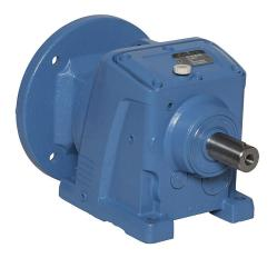
IronHorse heavy-duty helical gearbox, 30:1 ratio, 182/4TC-Face input, inline, 1.25in diameter output shaft, nominal 3hp at 1.0 SF, 3120 lb-in mechanical output torque, Type-47 frame, cast iron housing, foot mount.
